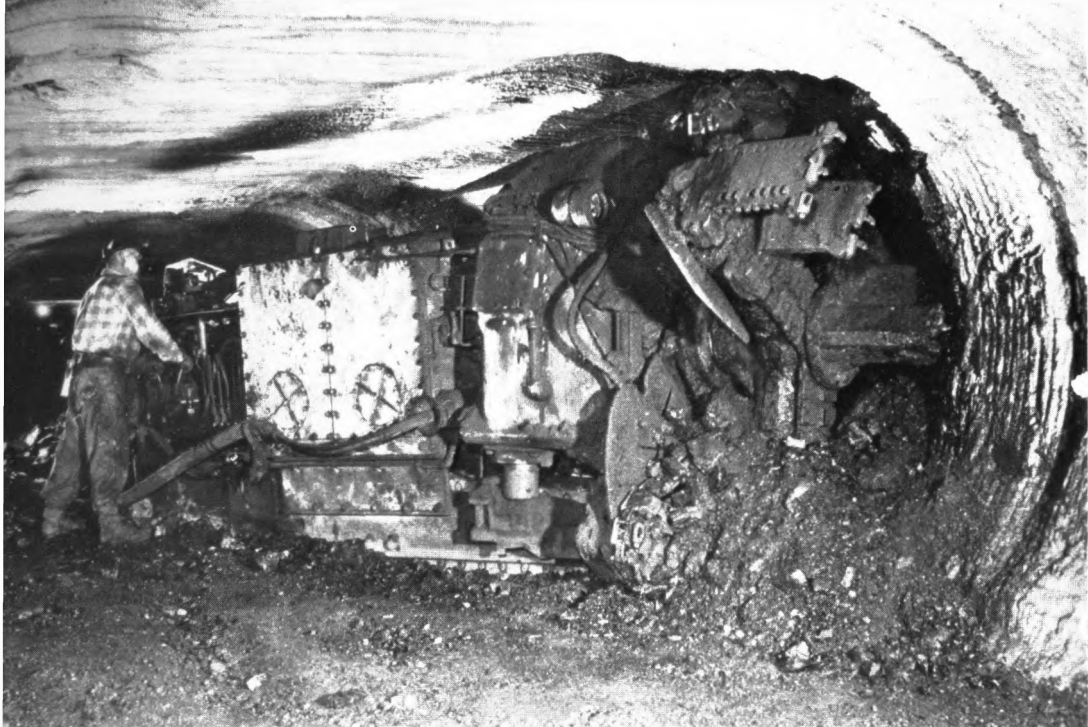
45 A power loader cutting and loading coal on to a conveyor belt, with self-advancing hydraulic supports on the left
